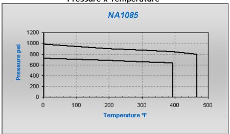
The P x T graph shown above indicates the service limits for this sheet considering pressure and temperature simultaneously...(Tests were performed with nitrogen on 1.6mm thick sheet). The "normal" curve represents the common usage area for this sheet while the "maximum" curve indicates the maximum limits. For applications near or above the "maximum" curve, contact TEADIT.
